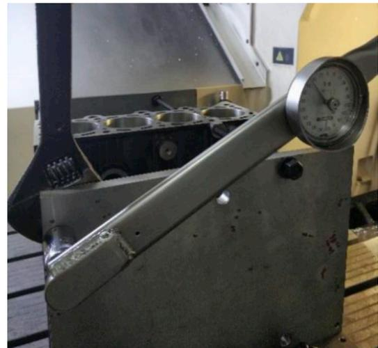
Fig. 26. Clamping force exertion by the torque wrench.
