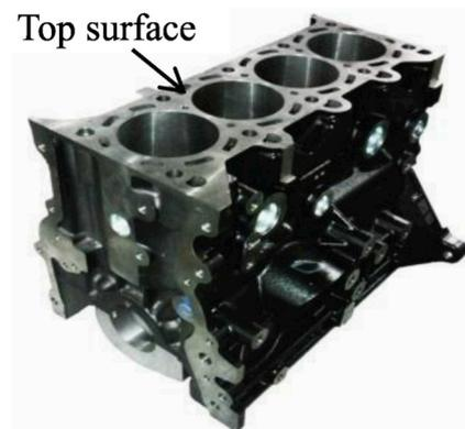
Fig. 18. A four-cylinder block of B12 engine.
